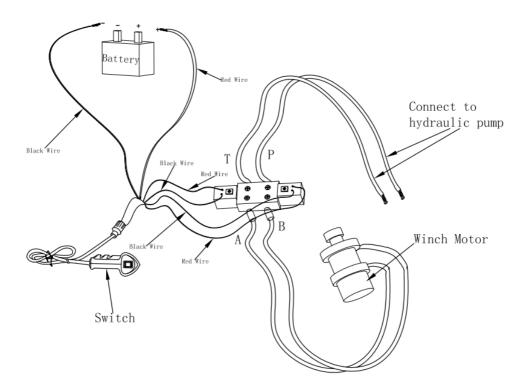
Fig 1. Basic Configuration Schematic
